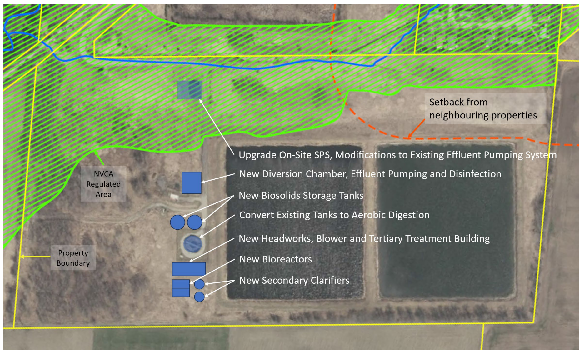
Figure 6.1 – Conceptual Layout for Design Concept Option 1 – Extended Aeration with Tertiary Filtration
